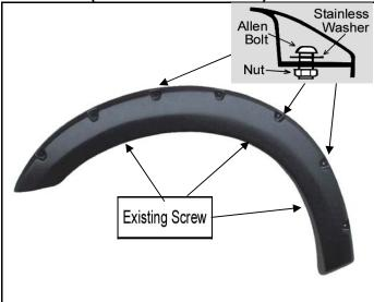
Use Torx Bit to tight allen bolt & nut firmly on every pocket of the fender flare, then place the flare on the vehicle with best position. Fasten the existing factory screws into the original location that were previously removed.
