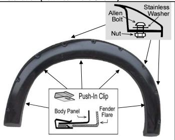
Use Torx Bit to tight allen bolt & nut firmly on every pocket of the fender flare, then place the flare on the vehicle with best position. Apply 5 Push-In Clip into the mounting slot in flare and secure it to the vehicle, as shown.
